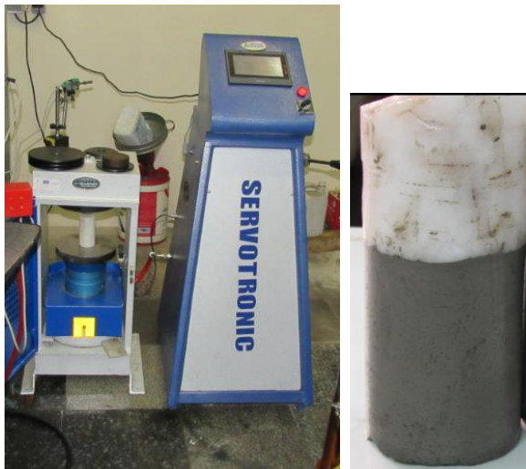
Figure 2. Sample prepared to determine the normal stiffness, with the uniaxial testing machine
