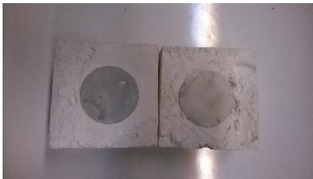
Figure 1. Samples prepared for shear tests with the direct shear machine
