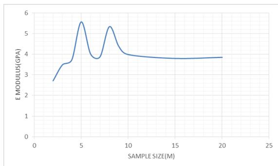
**Figure 7. Influence of sample size on the E modulus**
