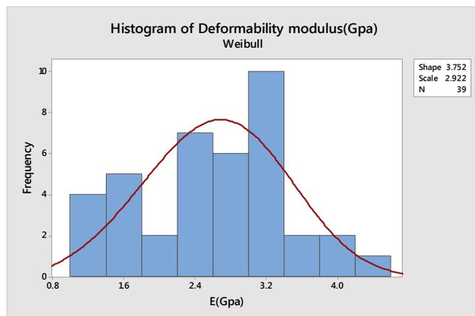
Figure 9. Deformability modulus value distribution
