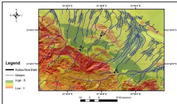
Figure 5. Finding 3 locations suitable for the construction of subsurface dams
