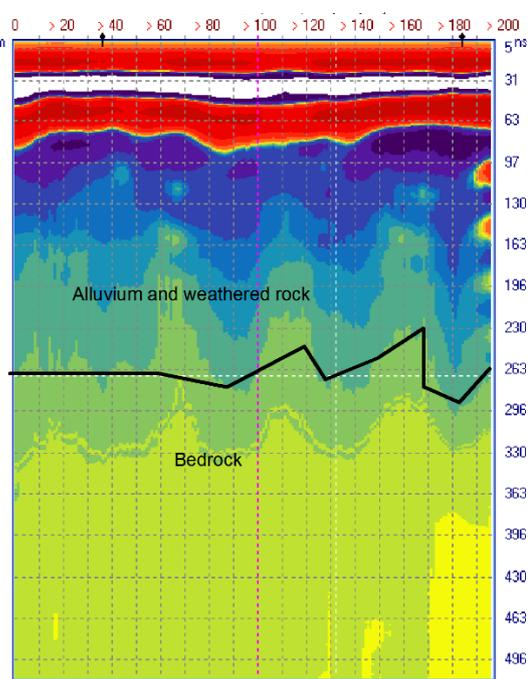
Figure 11. Georadar profile recorded and analyzed by Reflexw at location D3
