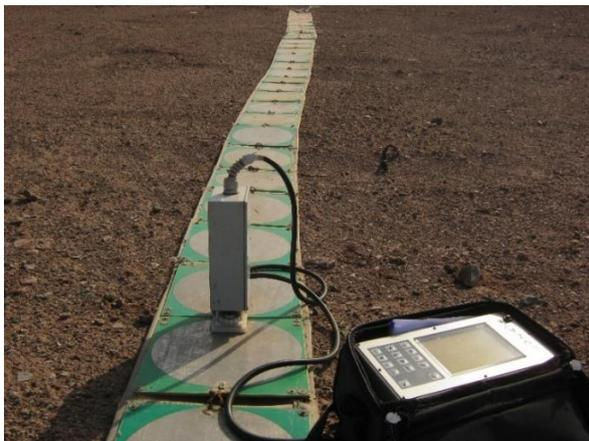
**Figure 1. Georadar complex Loza-M with 15 meters transmitters**
