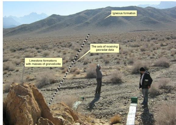
Figure 6. Given axis at location D1 to obtain the georadar data
