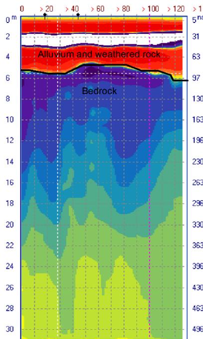
Figure 9. Georadar profile recorded and analyzed by Reflexw at location D2
