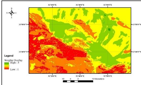
Figure 4. The map derived from the integration of effective layers in locating the subsurface dam
