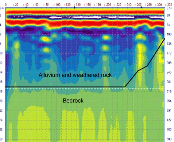
Figure 7. Georadar profile recorded and analyzed by Reflexw at location D1
