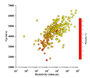
Figure 13. Relationship between P-wave velocity and electrical resistivity (porosity range indicated by color scale)
