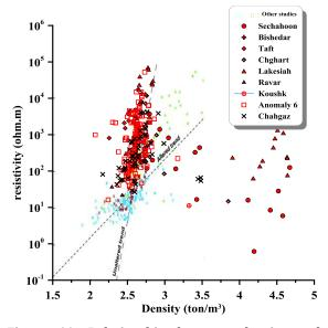
Figure 11. Relationship between density and electrical resistivity (compared with studies by Menier et al. 2020)
