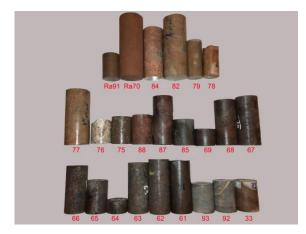
Figure 8. Samples containing magnetite and hematite minerals including samples of Ravar sandstone (Ra70, Ra91), samples of Lake Siah hematite mineral (61 to 69, 75, 87 and 88) and samples of Lake Siah dolomites (33,76, 77,92,93)
