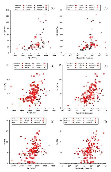
Figure 14. Relationship between mechanical properties and P-wave velocity and electrical resistivity, a and b) UCS, c and d) Tensile strength, e and f) point load index vs. P-wave velocity and electrical resistivity, respectively.
