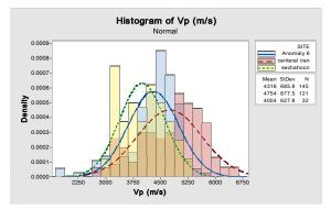
Figure 6. Statistical distribution of P-wave velocity of Anomaly VI, Sechahoon and other mines
