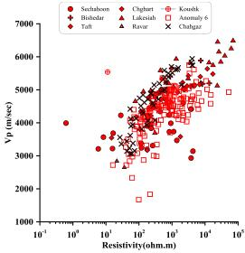
Figure 12. Relationship between P-wave velocity and electrical resistivity
