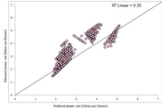
**Figure 9. Relationship between measured and predicted shearer rates in logarithmic non-linear multivariate regression using test data**
