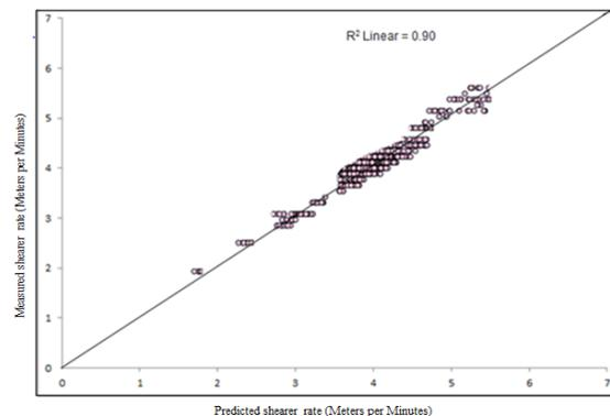
**Figure 4. Relationship between measured and predicted shearer rates in multivariate linear regression using training data**
