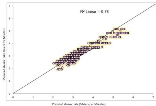
Figure 6. Relationship between measured and predicted shearer rates in exponential non-linear multivariate regression using training data
