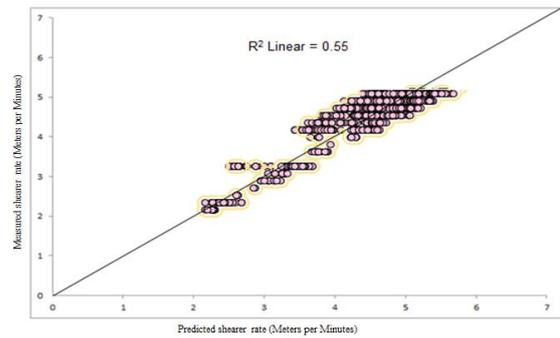
Figure 7. Relationship between measured and predicted shearer rates in exponential non-linear multivariate regression using test data
