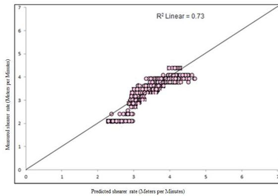
**Figure 5. Relationship between measured and predicted shearer rates in multivariate linear regression using test data**
