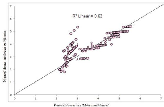
**Figure 8. Relationship between measured and predicted shearer rates in logarithmic non-linear multivariate regression using training data**
