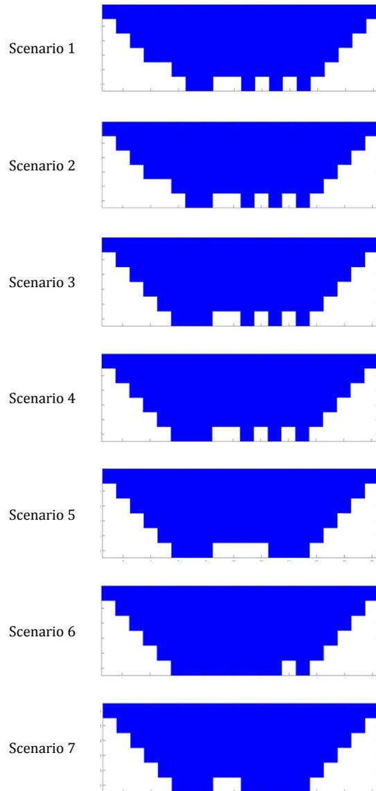
Fig. 3. The section view of the UPL shape of the block model in the east-west direction.
