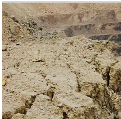
Fig. 2-. a) A sample of blasting and b) The undesirable backbreak after blasting in the Angouran mine
