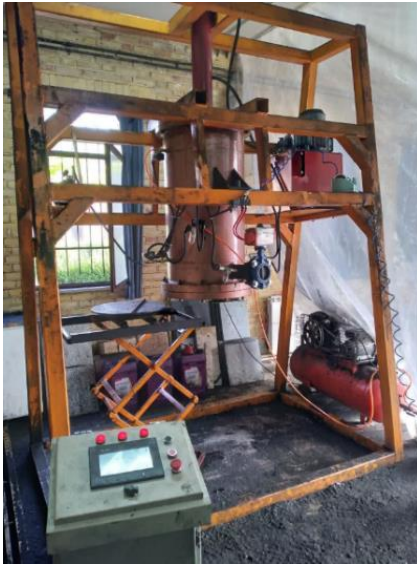
Fig. 5. A new device for investigating the phenomenon of instantaneous emission of coal gas and drainage of methane gas.
