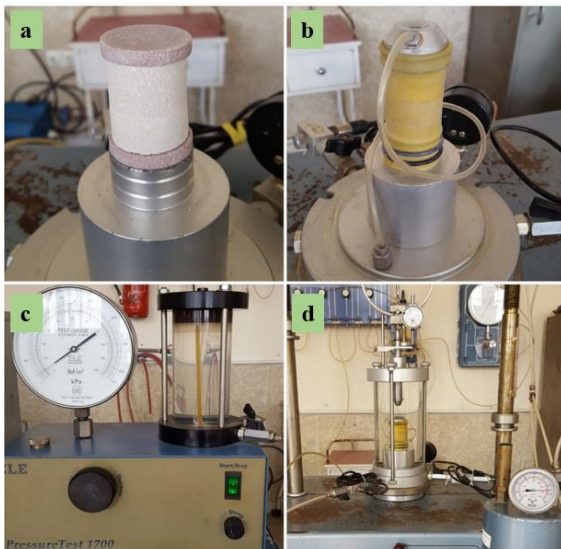
Fig. 7. The gas permeability testing setup: (a) created specimen, (b) specimen fitted in the gasket with the confinement, (c) the gas gauge, and (d) overlook of the setup.
