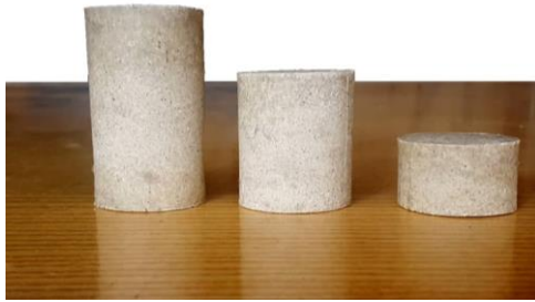
Fig. 4. The prepared cylindrical samples with 3.6 cm diameter and 2, 4, and 6 cm height.
