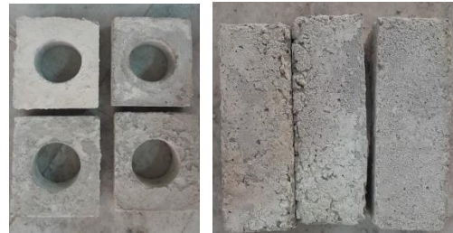
Fig. 4. Rectangular samples with a central hole
