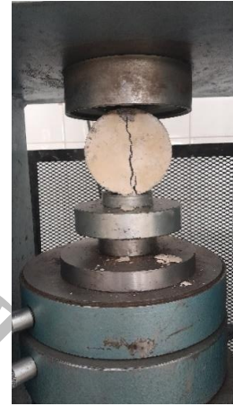
Fig. 1. Concrete sample under Brazilian test
