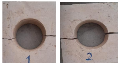
Fig. 12. Fracture mode of samples under direct tensile loading
