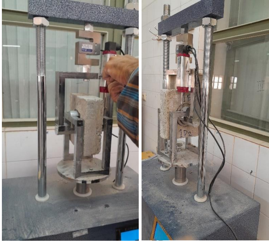
Fig. 3. The process of setting up the new apparatus based on the compressive to tensile load converter
