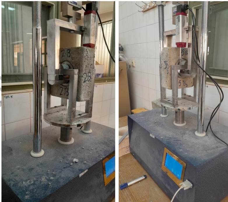
Fig 6. Rectangular specimen with a central hole under CTLTC loading
