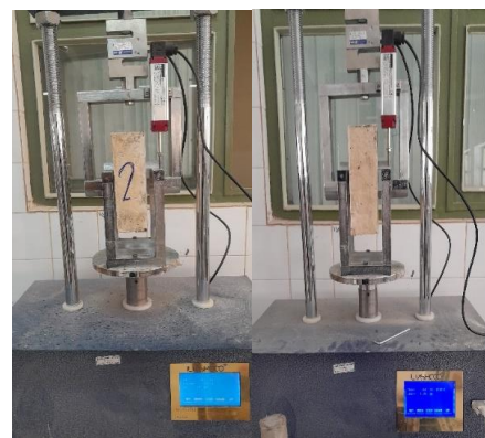
Fig. 11. Rectangular gypsum specimen with a central hole under CTLC loading
