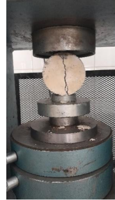
Fig. 1. Concrete sample under Brazilian test
