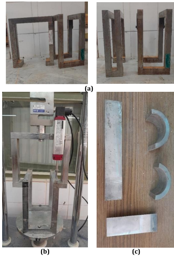
Fig. 2. Components of the compressive to tensile load converter (CTLC): (a) jaws for direct traction, (b) Cylindrical rods and loading steel circles, and (c) CTLC apparatus assembly
