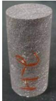
Fig. 1. A cylindrical rock sample according to the ISRM standard
