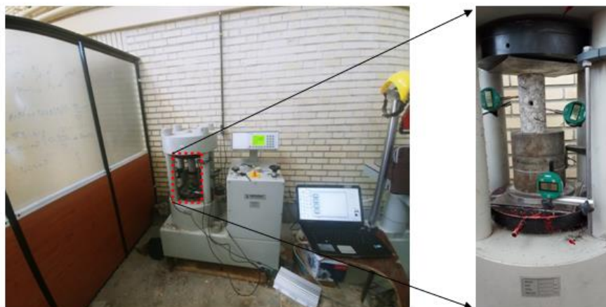
Fig. 10. Testing system (controlling laptop and Infra Test compressive strength with strain gauge)
