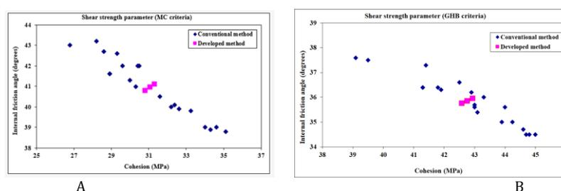
**Fig. 1: Comparison of shear strength parameters based on the conventional method and the developed method. A: the Mohr-Coulomb criterion, B: the Hoek-Brown criterion**
