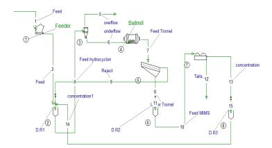
Fig. 1. The present (a) and the proposed flowsheets (b), for Iron processing in the Golgohar plant
