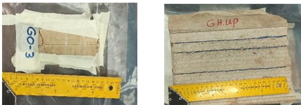
Fig. 1. Small-scale linear cutting test with a cutting depth of 2 mm on a rock sample.
