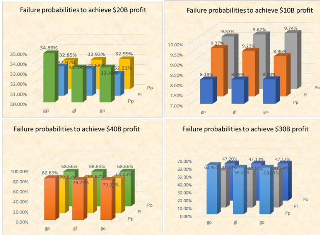
Fig. 1 . Diagram of the failure probability of nine pits according to different managerial objectives (Pp, Pl, and Po indicate pessimistic, logical, and optimistic prices, respectively, and gp, gl, and go indicate pessimistic, logical, and optimistic grades, respectively).
