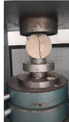
Fig. 1. Concrete sample under Brazilian test
