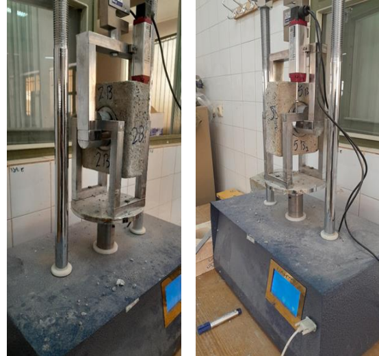
Fig. 6. Rectangular specimen with a central hole under CTLTC loading
