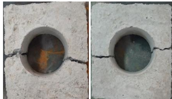
Fig. 7. Fracture mode of samples under direct tensile loading
