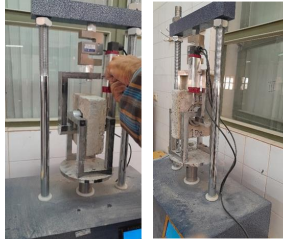
Fig. 3. The process of setting up the new apparatus based on the compressive to tensile load converter
