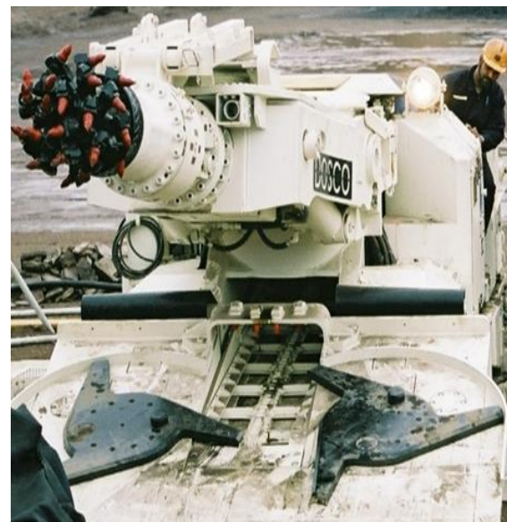
Fig. 2. A view of the Roadheader machine with axial excavation method in coal mines of Tabas [17].
