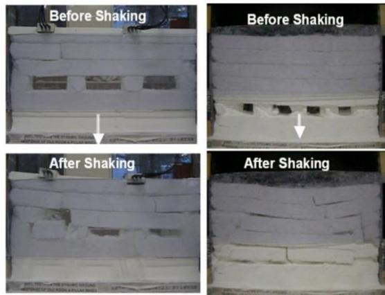
Figure 1. Physical model of a shallow (left) and deep (right) room and pillar mine subjected to the seismic load [5,9]
