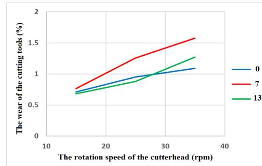
Fig. 8. The effect of the rotation speed of the cutterhead on the wear of cutting tools at 0, 7, and 13 % moisture contents.
