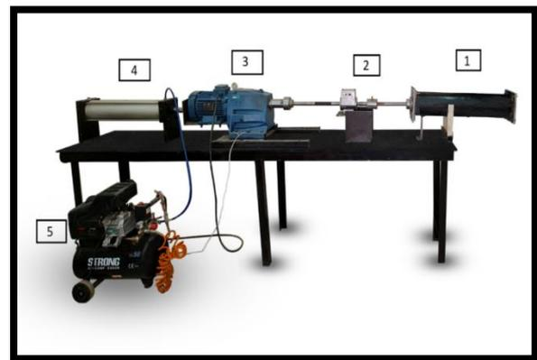
Fig. 1. Overview of the tunnel boring machine laboratory simulator, 1- shaft and excavation chamber, 2- torque meter, 3- motor and gearbox, 4- pneumatic jack, and 5- air compressor.
