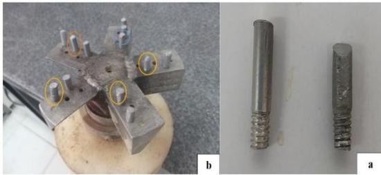
Fig. 9. a). The cutting tool with the highest and the lowest wear, b). the worn surfaces of the tools installed on the tunnel boring machine laboratory simulator.
