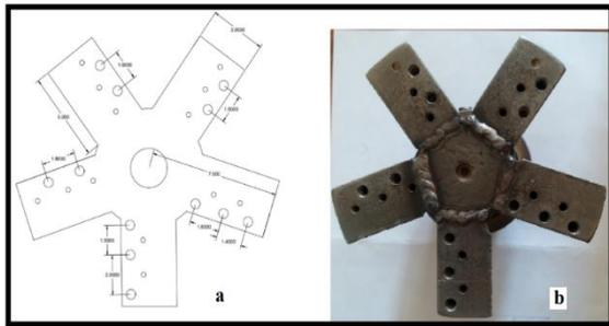
Fig. 4. a) Two-dimensional view of the cutterhead drawn in AutoCAD, b) Constructed cutterhead.
