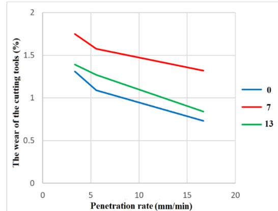
Fig. 10. The effect of the penetration rate on the wear of cutting tools at 0, 7 and, 13 % moisture contents.
