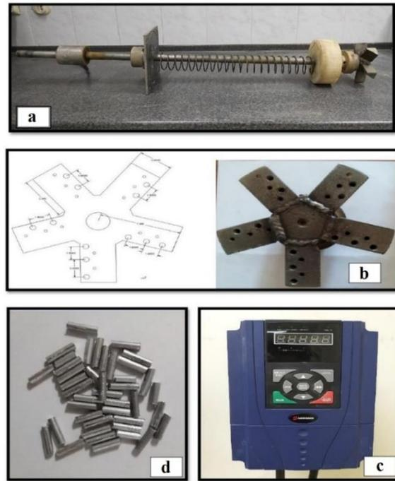
Fig. 2. a) A view of the shaft and cutterhead set, b) Cutterhead of the tunnel boring machine laboratory simulator, c) The device for adjusting the rotation speed of the cutterhead, d) Aluminum pins (cutting tools) used in the experiments.
