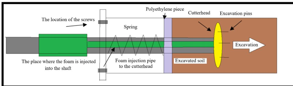
Fig. 3. A schematic view of the shaft of constructed excavation machine and its soil chamber.
