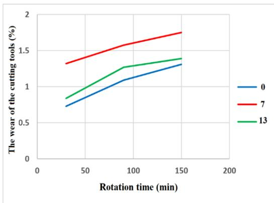
Fig. 10. The effect of the rotation time on the wear of cutting tools at 0, 7, and 13 % moisture contents.
